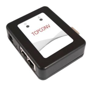
The main purpose of the TCP converters is to enable RFID authentication and access control for devices that lack a USB port, from older single function printers to industrial robotics.
